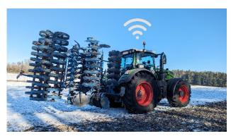
Even the control of the rear hydraulics for coupling implements (here a disc harrow) can be controlled remotely using Arnold NextG technology.
