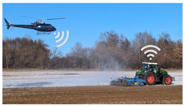
This Fendt 942 Vario has been equipped with a redundant electronic steering and driving system from Arnold NextG and can therefore be teleoperated or driven remotely - even from a helicopter.
