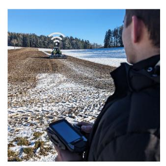
The digitalization of previously manual or hydraulic vehicle functions makes it possible to operate the Fendt 942 Vario by remote control - without a human driver in the cab.
