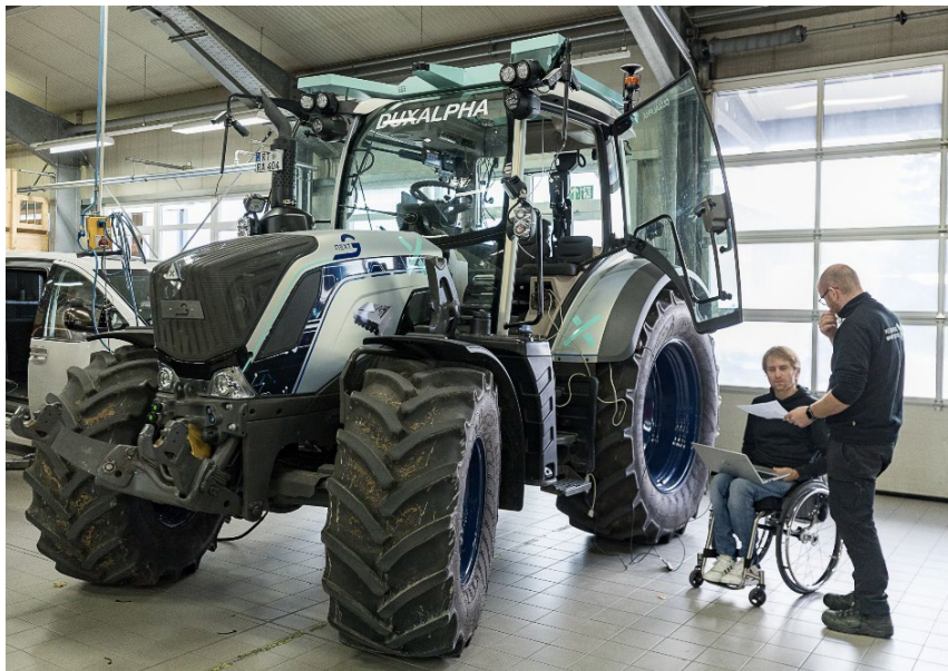
High tech meets practical application: This tractor has been prepared for teleoperation and is equipped with sensors and camera systems. It is fitted with the NX NextMotion drive-by-wire system and the DuxAlpha 3D guidance system for autonomous field work during system configuration. Photo: Arnold NextG
