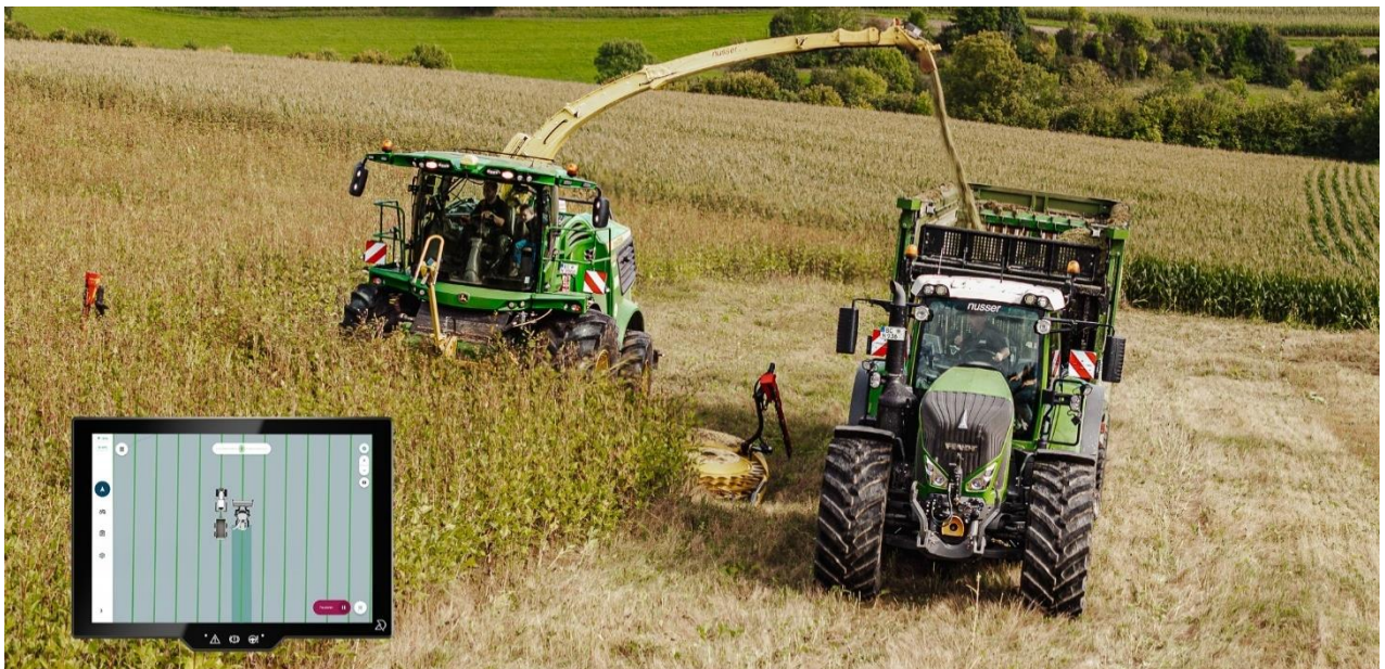
Autonomous operation: The NX NextMotion system takes over the digital control of the tractor, while the DuxAlpha system handles 3D guidance and the coordination of the machine fleet, ensuring precise workflows even on sloping terrain. Photo: Arnold NextG
