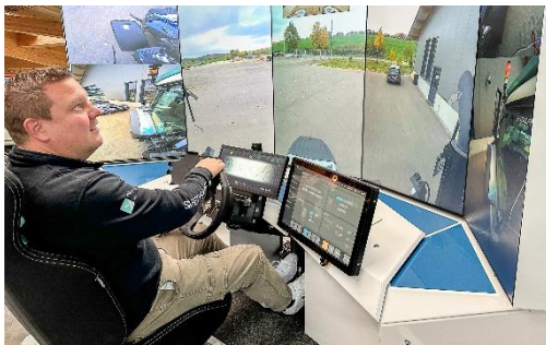
Take a look inside the control centre: The teleoperator controls the tractor remotely via a multiscreen visualisation system, sensor feedback and a digital cockpit. Photo: Arnold NextG
