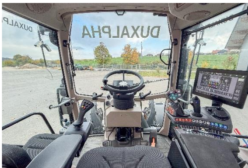
In action: The tractor is operated remotely. The camera image replaces the view from the cab and all control and system monitoring is carried out from the control centre. Photo: Arnold NextG
