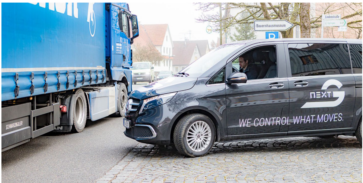
Remote-controlled driving in a real-world environment: An NX NextMotion-equipped V-Class test vehicle travels independently on public roads. It is controlled from a control centre via a multi-redundant drive-by-wire system that controls steering, braking and propulsion. Photo: Arnold NextG
